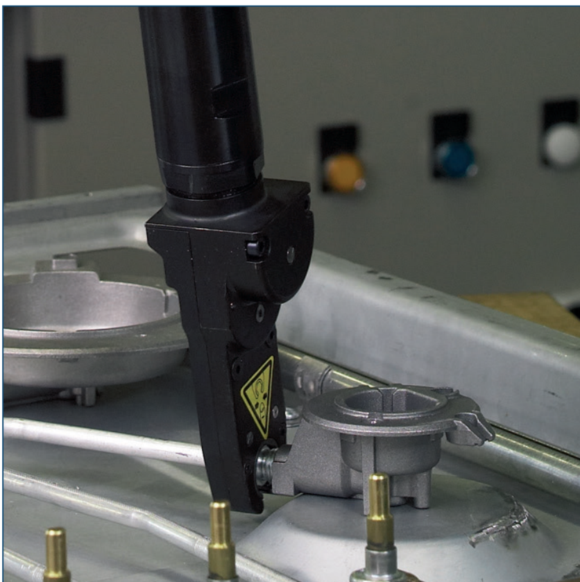
Radial opening ideal to reach the nut.
