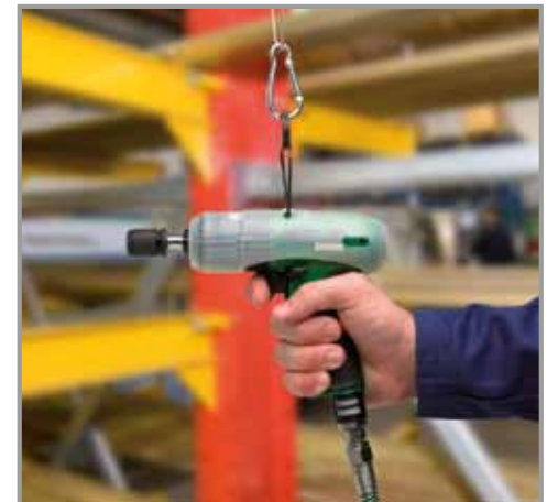
Models with pneumatic pick-up signal (ported) for screw counting (poka yoke system) available upon request
