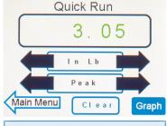
Use Quick Run mode to perform a single run torque test and view a graph of the results.
