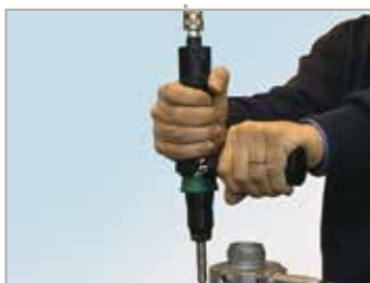
Air screwdrivers with auxiliary grip.
